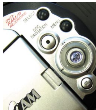
Fig. 4—Joystick as Navigation Interface Applied for DVD Camera for First Time.
