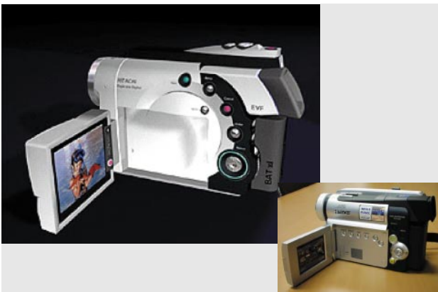
Fig. 6—Virtual 3D Rendering and Animation on PC. Real 3D Model for Final Evaluation. Designers will deliver 3D technical drawing to the engineering department for physical 3D models realization to be applied for engineering moulds in various materials.
