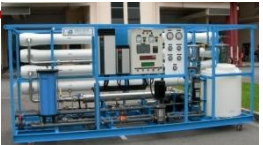
RO membrane water treatment
